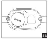
2. Using a fingernail or small object such as a ball point pen, push the gold battery clip out then remove the battery.
