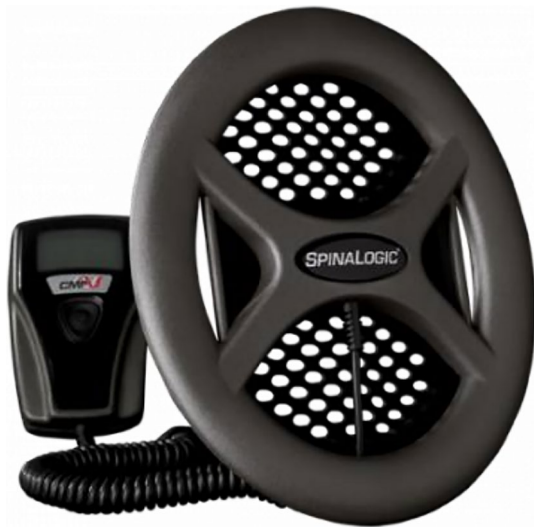
Fig. 1 SpinaLogic ® bone growth stimulator. The electronic control module and the transducer coil are depicted. The module includes a signal generator that produces an electrical signal which is transmitted to the treatment transducer. The transducer coil is an elliptically shaped copper wire coil that converts the electrical signal into an electromagnetic field
